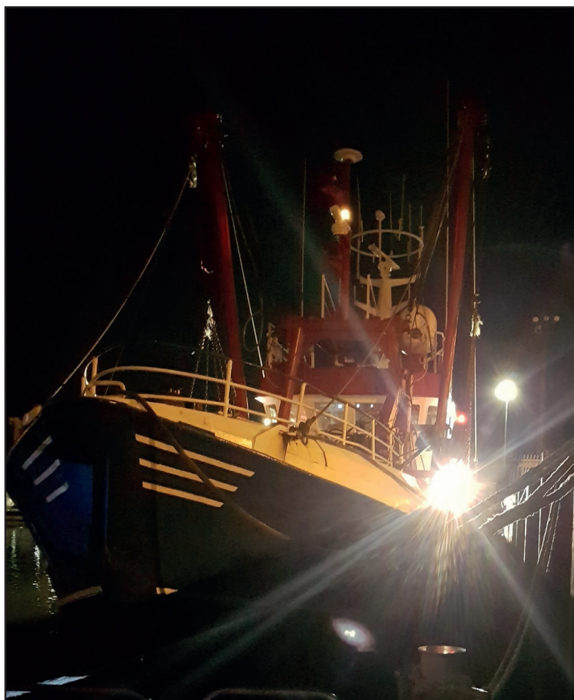
Figure 6: Vertrouwen 's forward facing dredge deck floodlights visible from ahead
