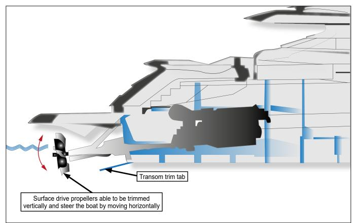
Figure 6: Diagram of Vision's surface-drive propulsion system
