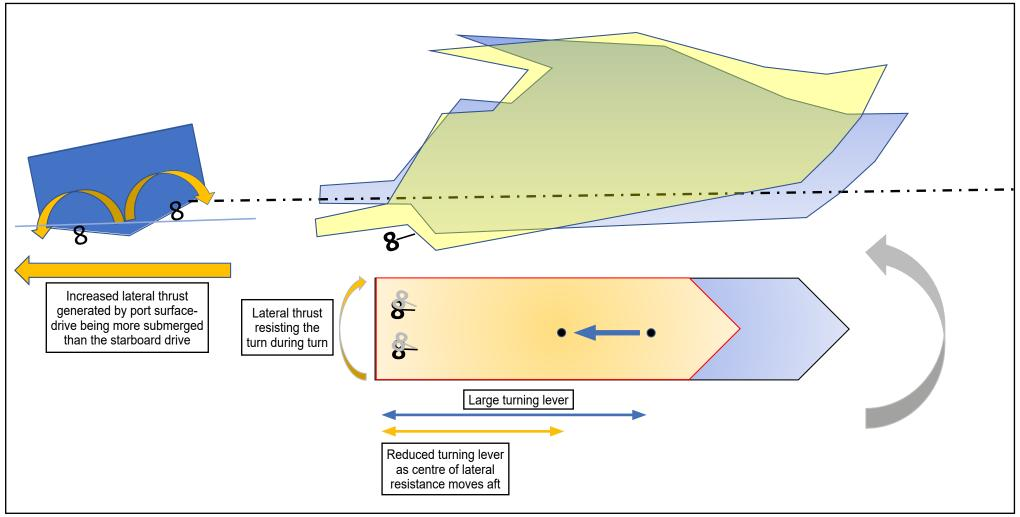
Figure 8: Factors affecting Vision's manoeuvrability immediately prior to collision
