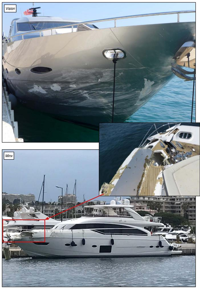
Figure 5: Detail of damage to both vessels
