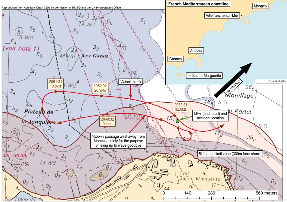
Figure 3: Vision's track derived from AIS data with times and speeds shown
